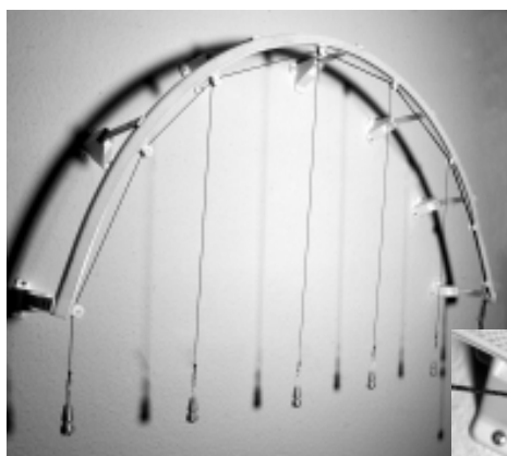
RPS mountboard and rollers used in an arched window
